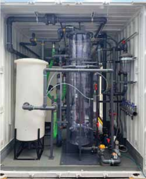
Foam fractionation pilot-scale system, Syracuse, New York
