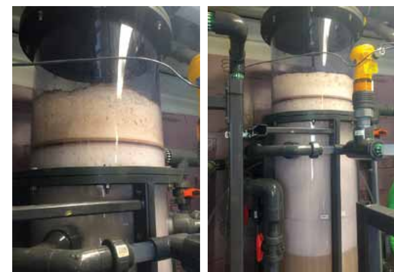
Foam fractionation pilot system foam generation: in collection cup head (left), in column (right)
