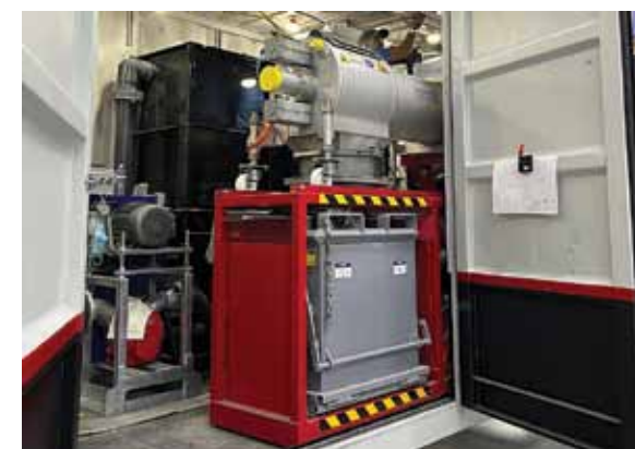
Figure 6. SCWO demonstration system planned for Orange County, California. (top) water-phase diagram Photo courtesy of 374Water
