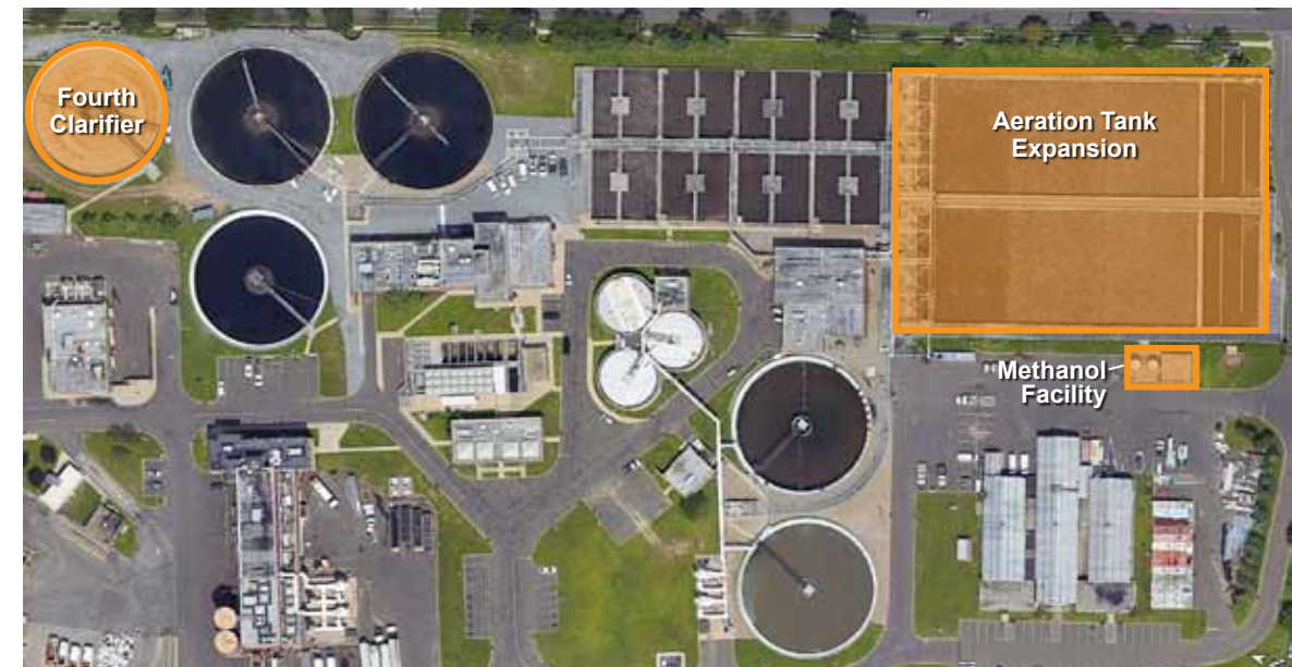
Figure 2. Stamford WPCF 2004 upgrade/expanded facilities
