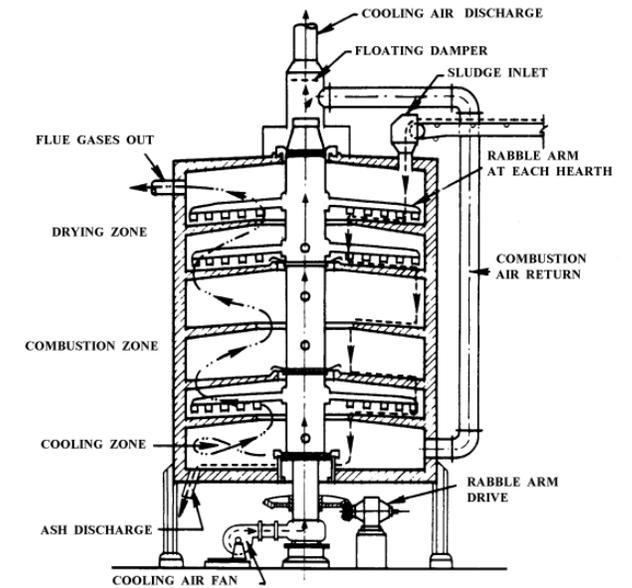
Cross section of a multiple hearth furnace
