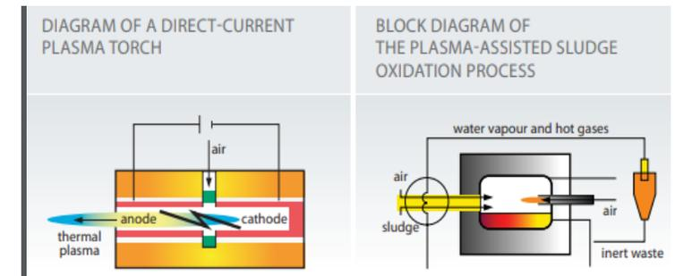
**Plasma-Assisted Sludge Oxidation**
