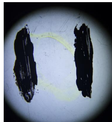
Photo by Author Fig. 2 Immobilized glucose oxidase on graphene with conductive paint.
