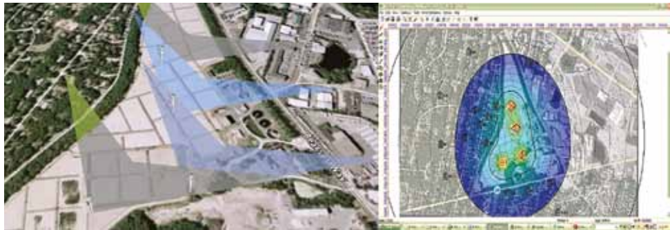
Figure 4. Wind turbine flicker study and sound level analysis results (showing the initial plan for four 225-kW turbines)
