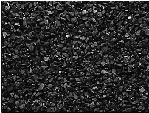
Granular Activated Carbon (GAC)
