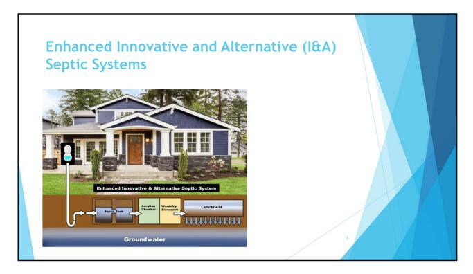
Enhanced I/A is the new generation with performance at or better than 12mg/L effluent nitrogen.
