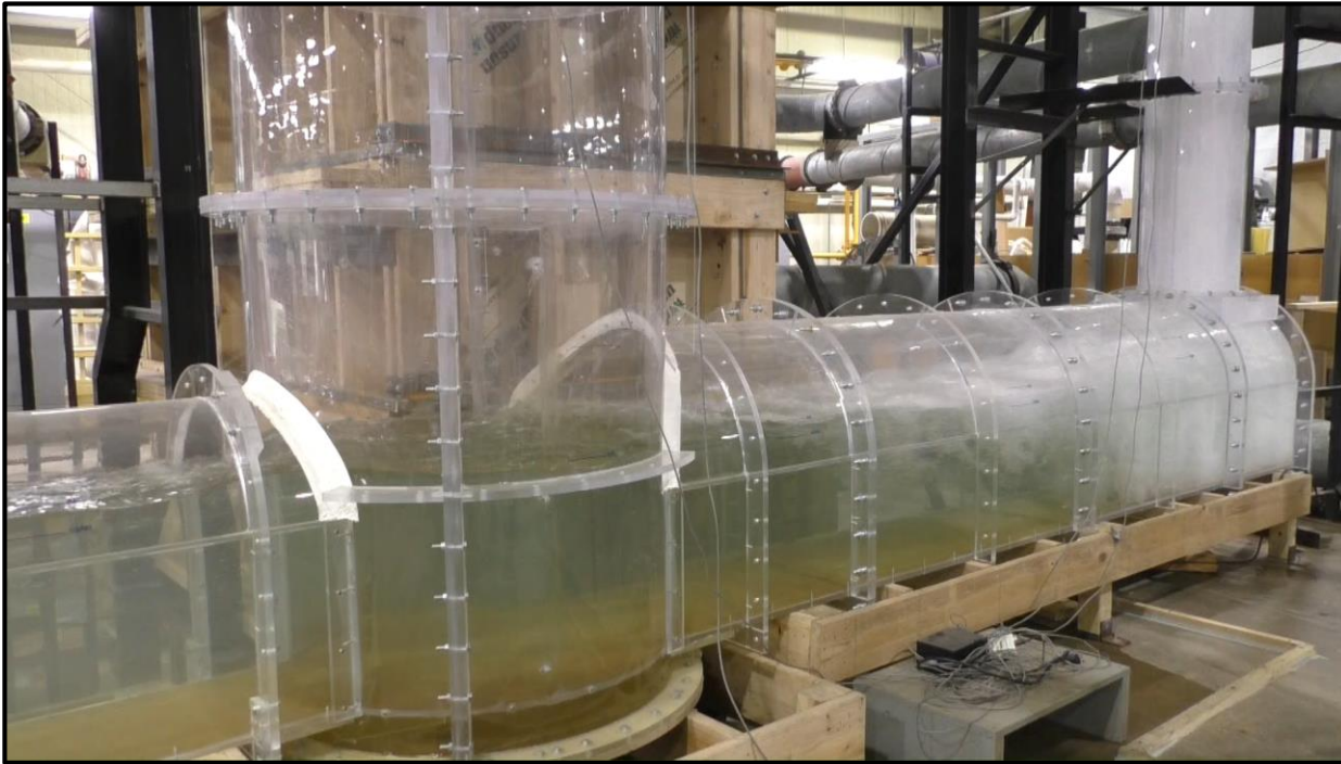
Papillon Drive Plunge Drop Shaft and Deaeration Chamber
