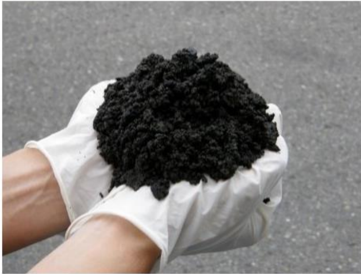
dewatered biosolids at 22% ds
