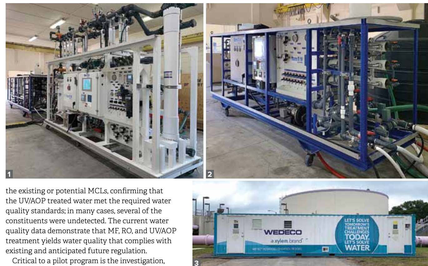
Figure 3. Plant City pilots 1. MF, 2. RO, 3. UV/AOP
