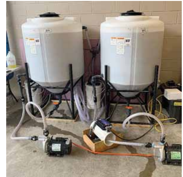
The pilot is testing a portable device meant to extract high-strength phosphorus from wastewater
