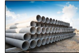
Asbestos Cement Pipe
