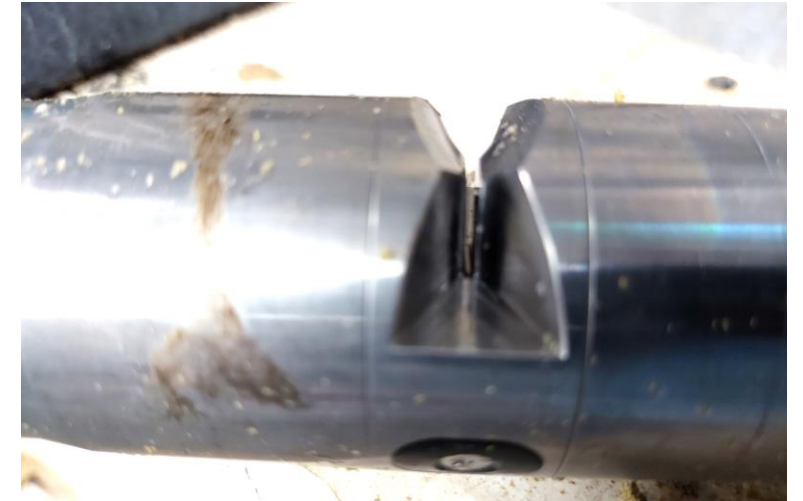
Sensor measurement window, 1 month since last cleaning
