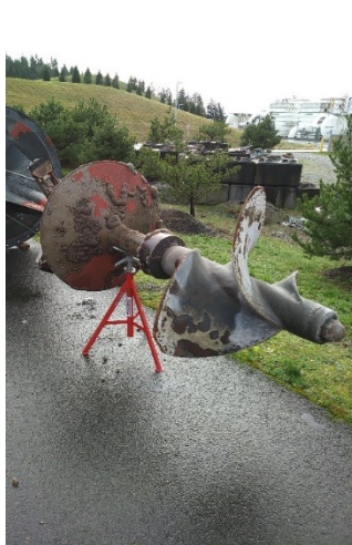
Draft tube mixer fouling
