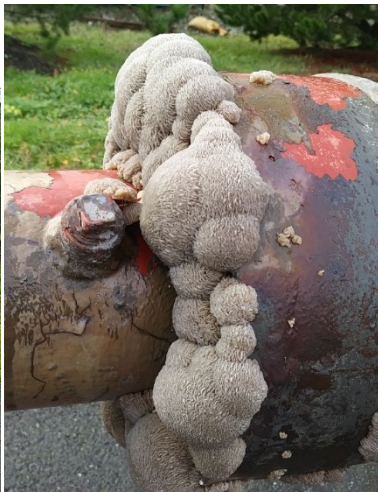
Draft tube mixer fouling
