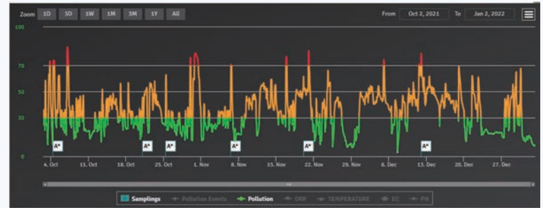
Graph: Pollution level as measured by Kando's system. Samples are collected and analyzed at the lab when the pollution is high (red)
