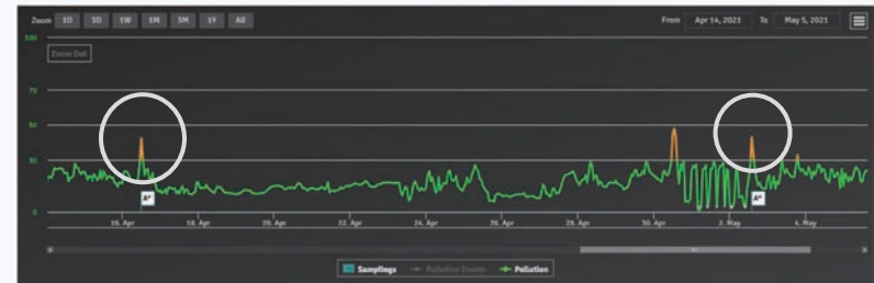
Graph: Pollution over time as seen in Kando Pulse., including 2 peaks where lab results indicated elevated levels of ammonia.
