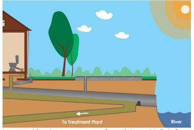
In a combined sewer, sewage from sinks and toilets flows to the treatment plant during normal (dry) conditions.
