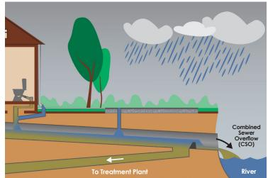
During heavy rains, CSO outfalls act as relief points to alleviate surface flooding and system backups by releasing excess sewage and stormwater to local waterbodies.
