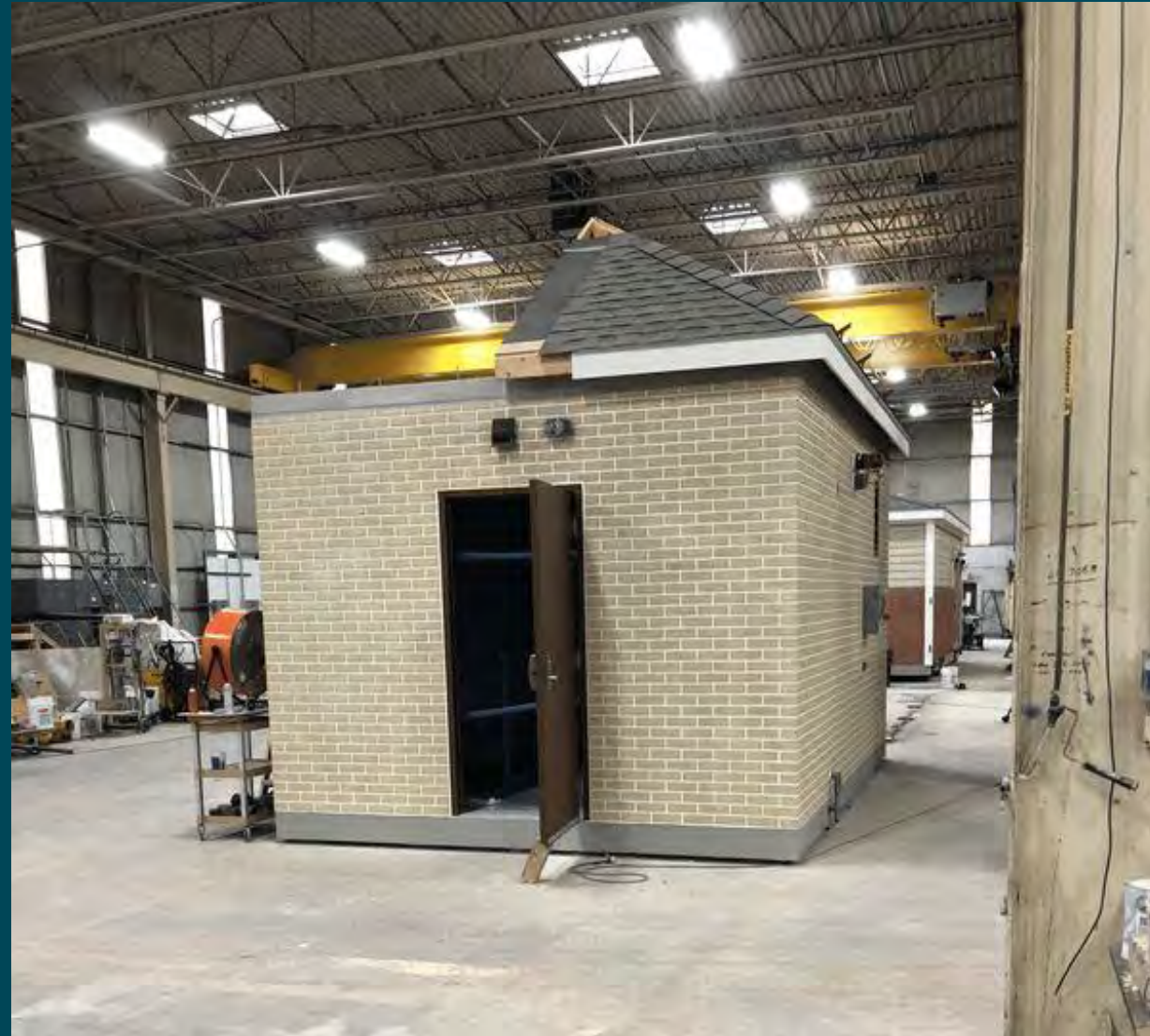
Pump Station Superstructure at United Concrete Factory
