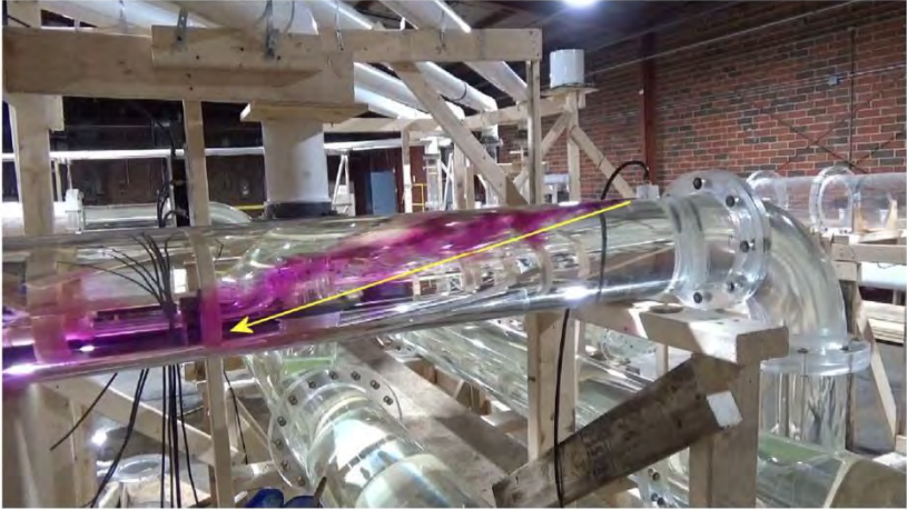
Photo 5-1 Flow Starts Circulating After Existing Elbow (long pipe)
