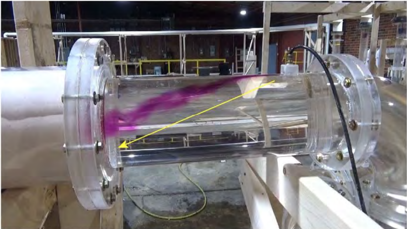
Photo 5-2 Flow Starts Circulating After Exiting Elbow (short pipe)
