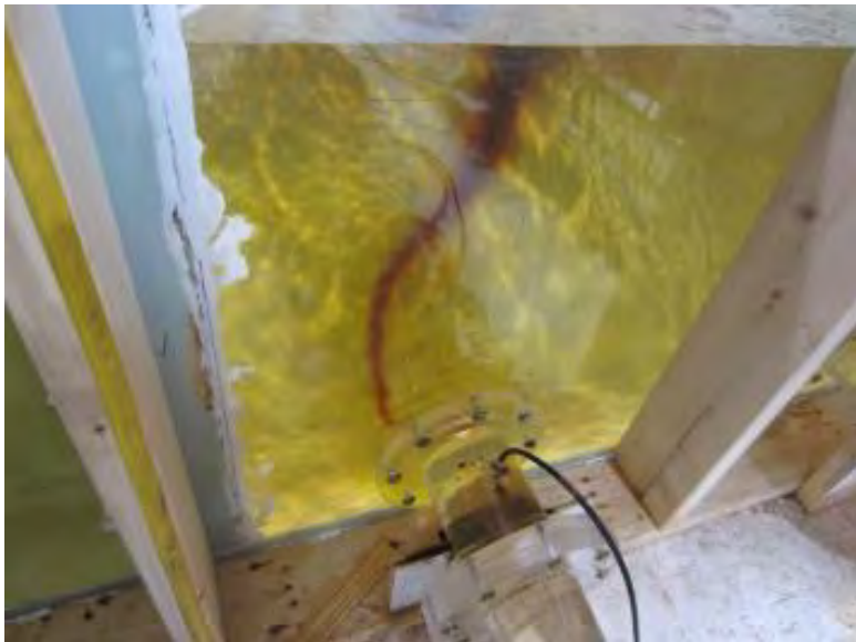
Vortices Forming with Existing Intake Arrangement
