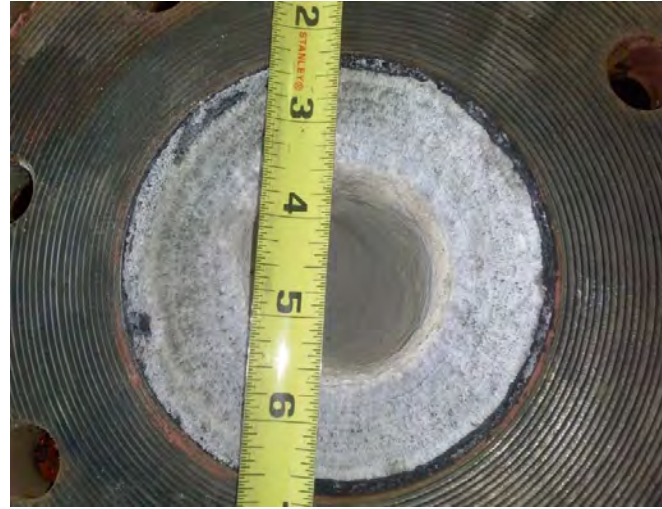
Struvite growth in pipe. ID decreased from ~4" to 2"
