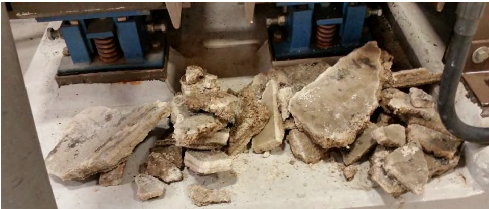
Struvite build up on pump impeller after just 15 days
