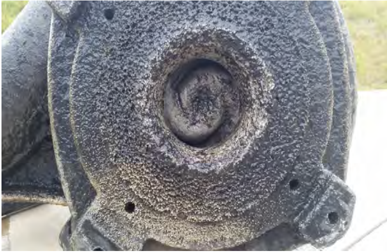
Struvite build up on pump impeller after just 15 days
