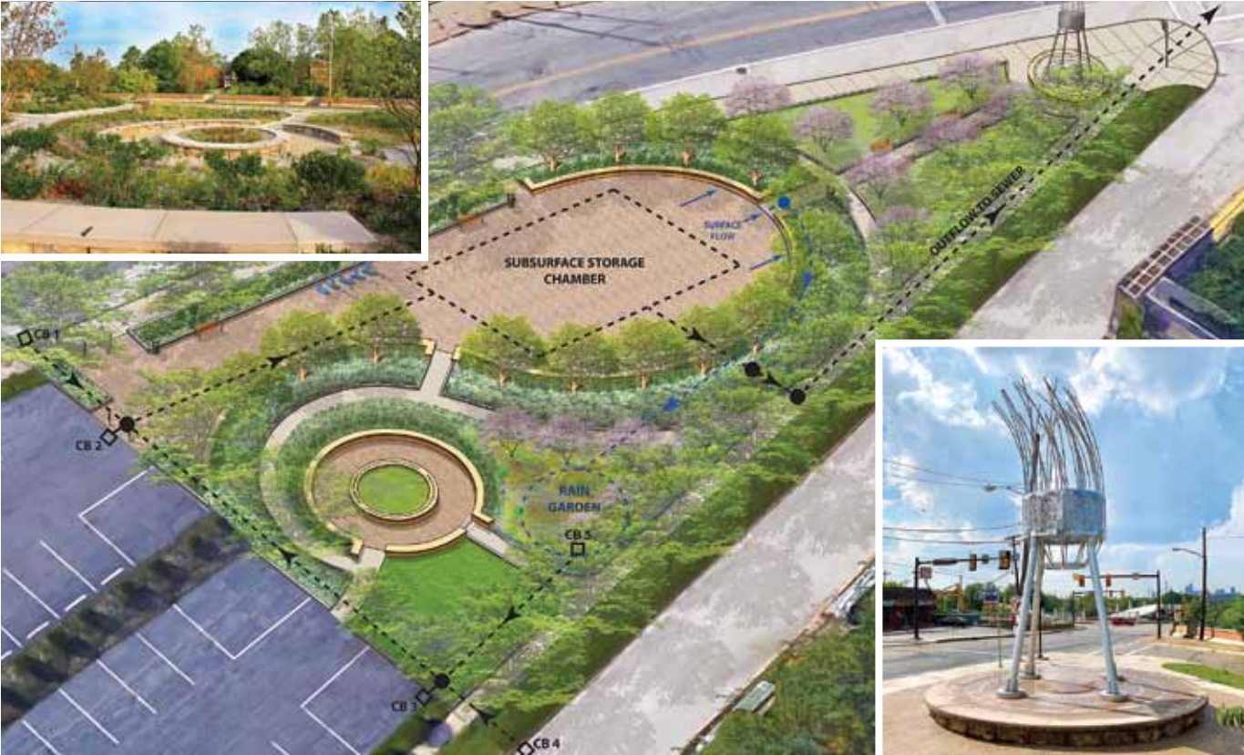
Figure 4. The Buckeye neighborhood Gateway site utilizes subsurface chambers for stormwater storage. Impervious areas throughout the site drain to a demonstration rain garden (top insert). An abstracted water tower sculpture is a focal point
