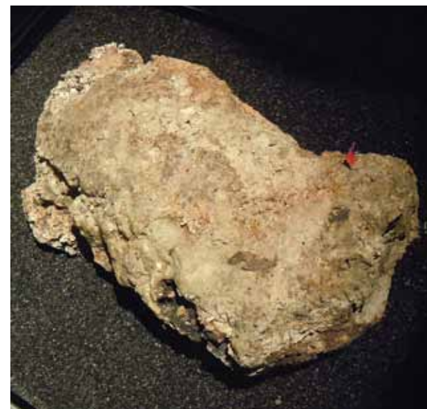
A dried section of a “fatberg” removed from the sewers of London
