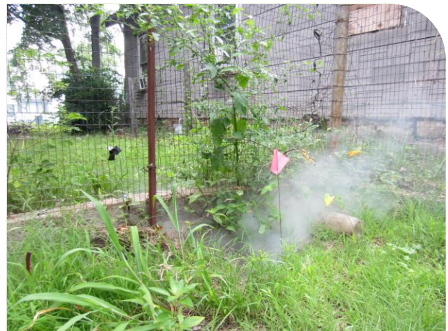
Smoke testing is used to detect sources of I/I. Image by Tetra Tech
