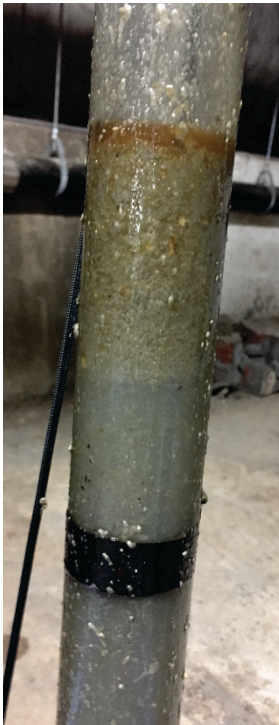
Figure 5-1 – Interceptor “core” sample using “sludge judge”
