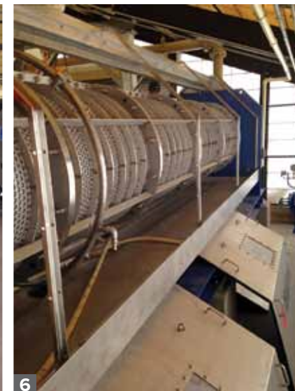
5. Installed grinder and plunger pumps 6. Screw press with cover panels removed showing the basket and washwater spray bar 7. Container (30 yd 3 ) (23 m 3 ) with leveling cover and conveyors and screw press in background
