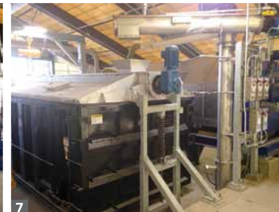
5. Installed grinder and plunger pumps 6. Screw press with cover panels removed showing the basket and washwater spray bar 7. Container (30 yd 3 ) (23 m 3 ) with leveling cover and conveyors and screw press in background
