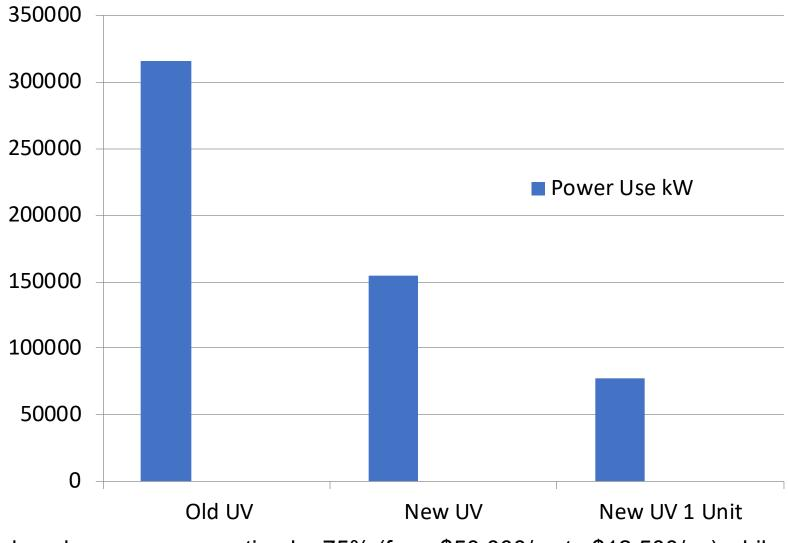
Reduced power consumption by 75% (from \$50,000/yr. to \$12,500/yr.) while maintaining disinfection limits.
