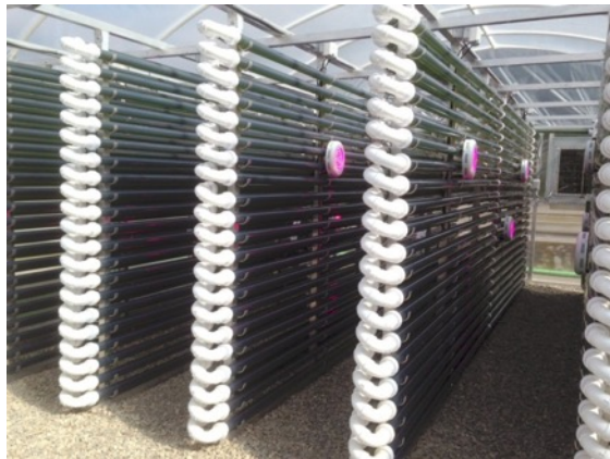
CO 2 Addition and Photobioreactor with LED Lights
