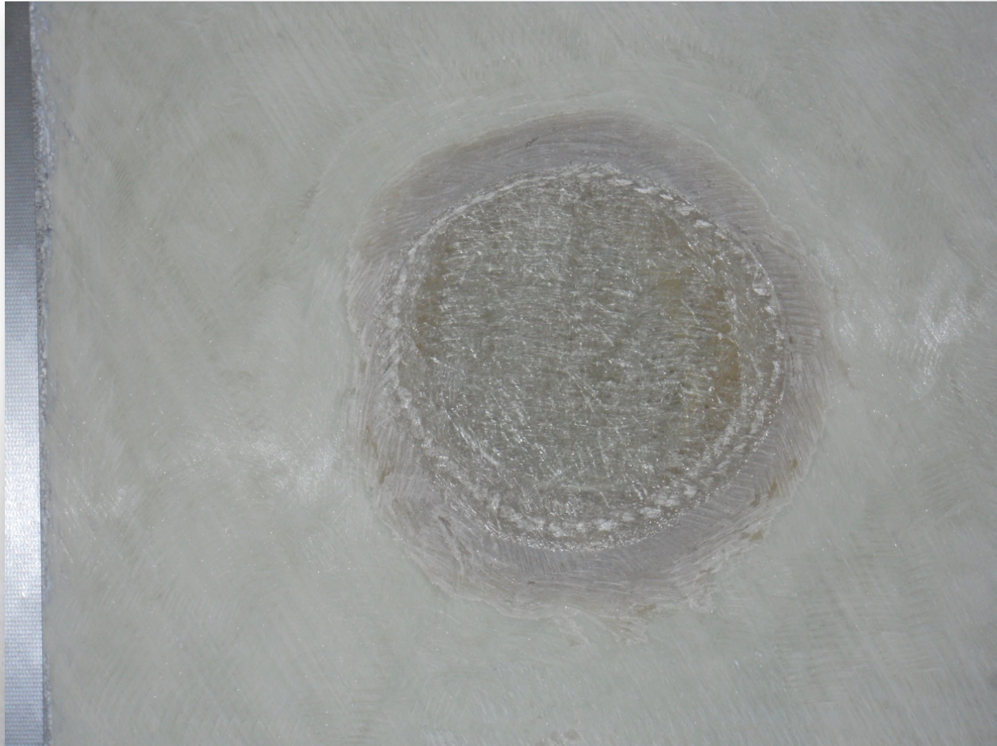
Shows the RFP repair prior to white resin gel coating – Sample Area
