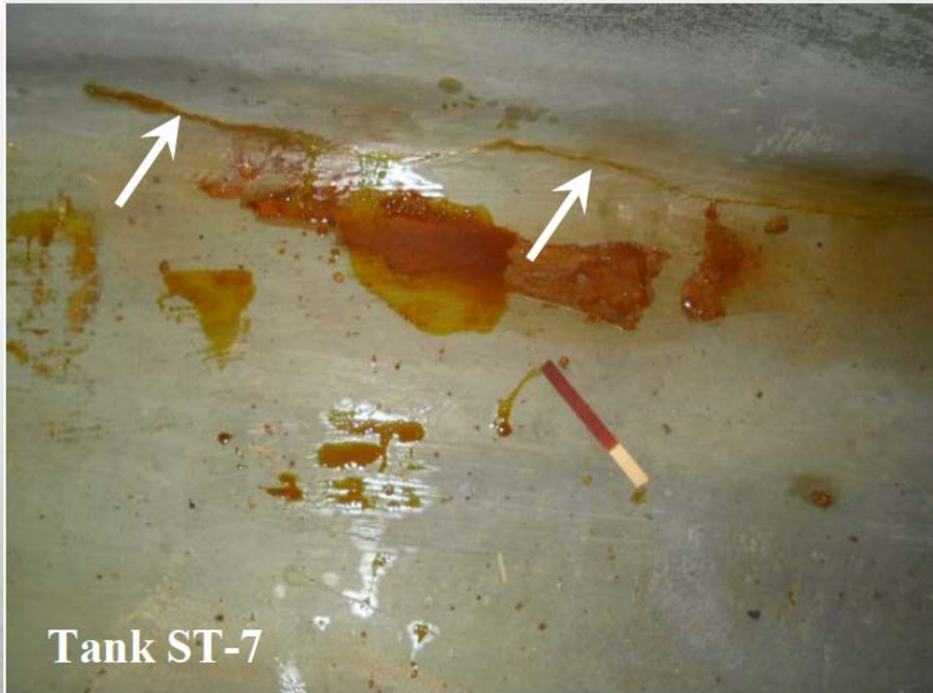
Cracking of corrosion barrier where floor laminate was applied over balsa core
