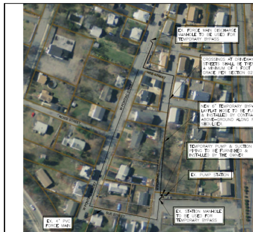
TEMPORARY BYPASS PUMP PLAN SCALE: 1"=50'-0"
