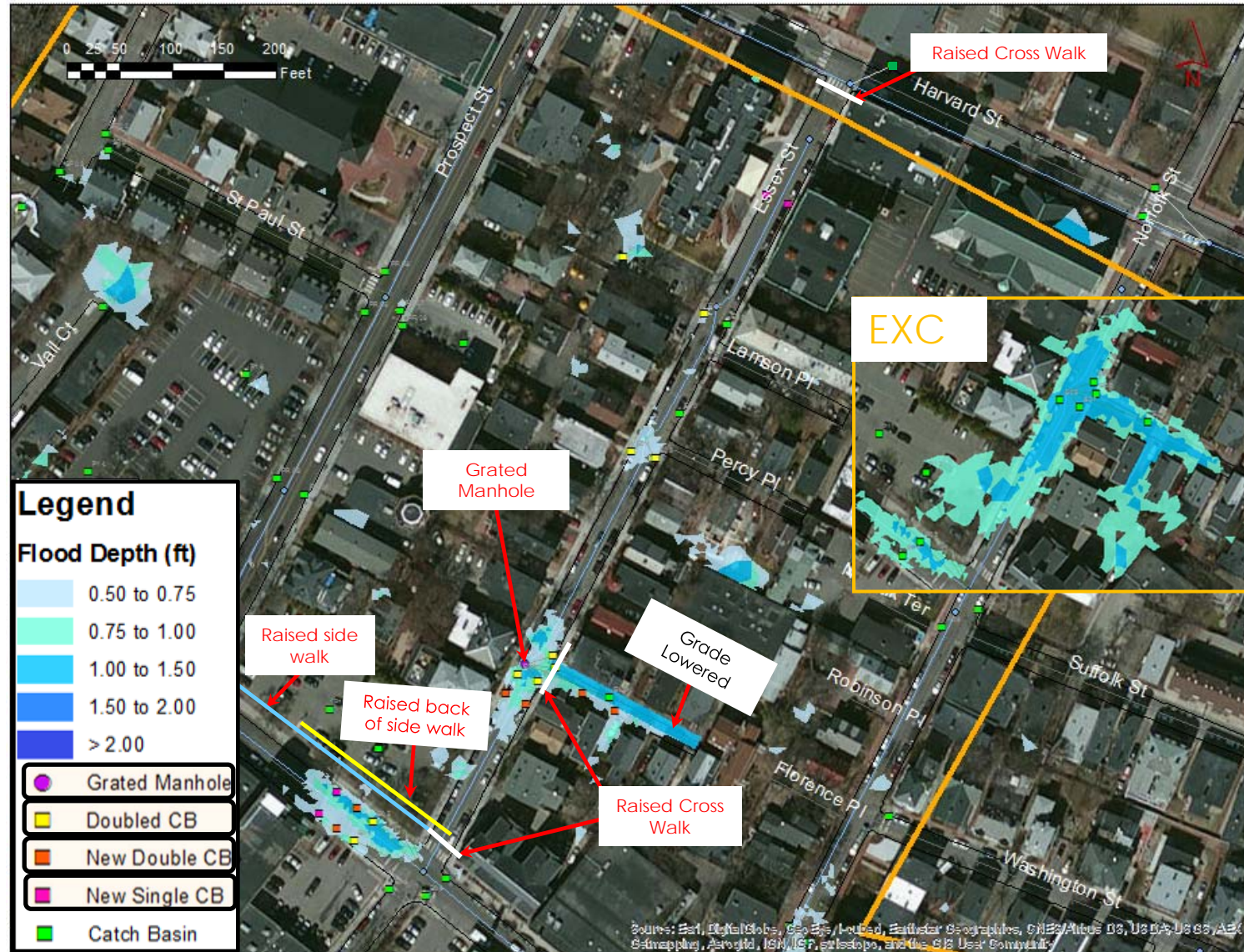
Simulated ground surface flooding during the 1.5 in/hour – 1 hour design storm under Proposed Conditions
