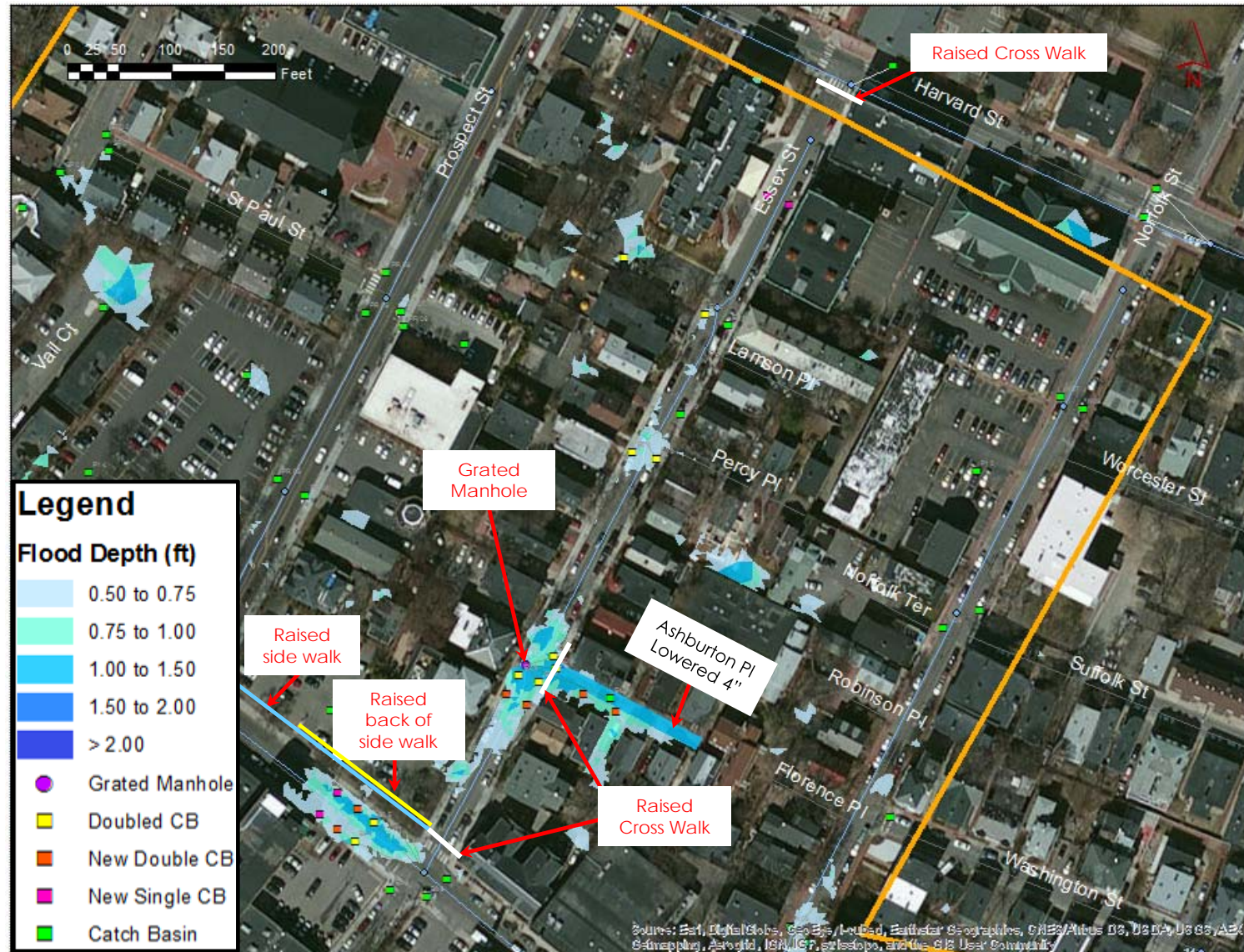
Simulated ground surface flooding during the 2.5 in/hour – 30 min design storm under Proposed Conditions
