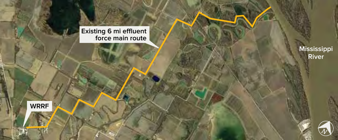
Figure 4. Location of O’Fallon WRRF and effluent force main to Mississippi River
