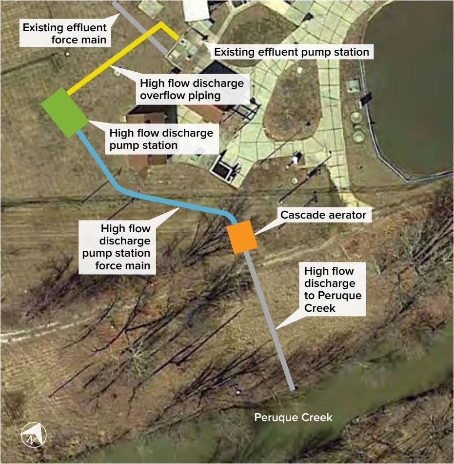
Figure 5. Proposed high flow discharge site plan
