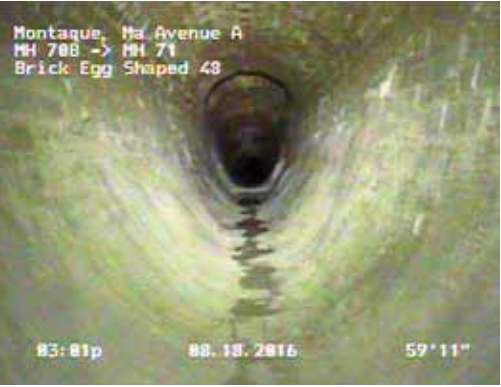
Photo 2. Rehabilitated upper drain invert restored to original shape
