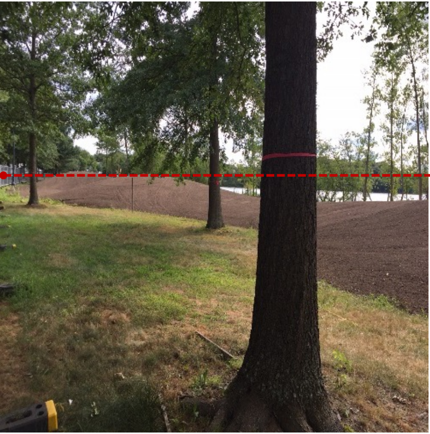
Build a vegetated berm at elevation 23.1 ft-CCB ( Cambridge city-based datum ) along Fresh Pond. This strategy could protect the Fresh Pond Reservoir for the projected 2070 100 year sea level rise / storm surge flooding.
