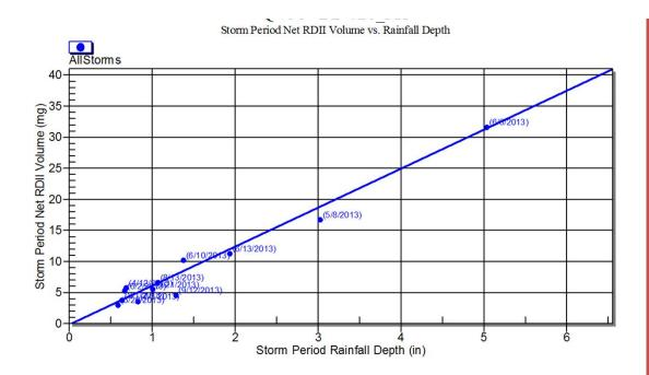
Q vs i is a linear relationship. Poor correlation coefficients are usually due to insufficient rain data. Each data point represents a storm.
