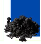
**CoMag®-** Ballasted Flocculation with Magnetite, by Evoqua Water Technologies
