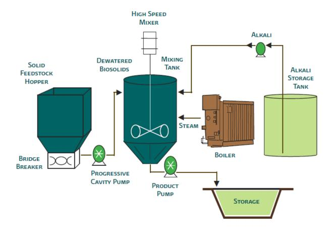
A Single Reactor Can Process 12-15 WT Per Hour
