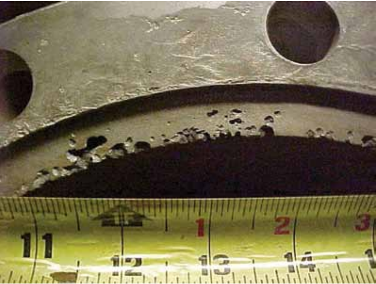
Figure 6. Typical crevice corrosion damage at a flanged connection due to chloride ion concentration
