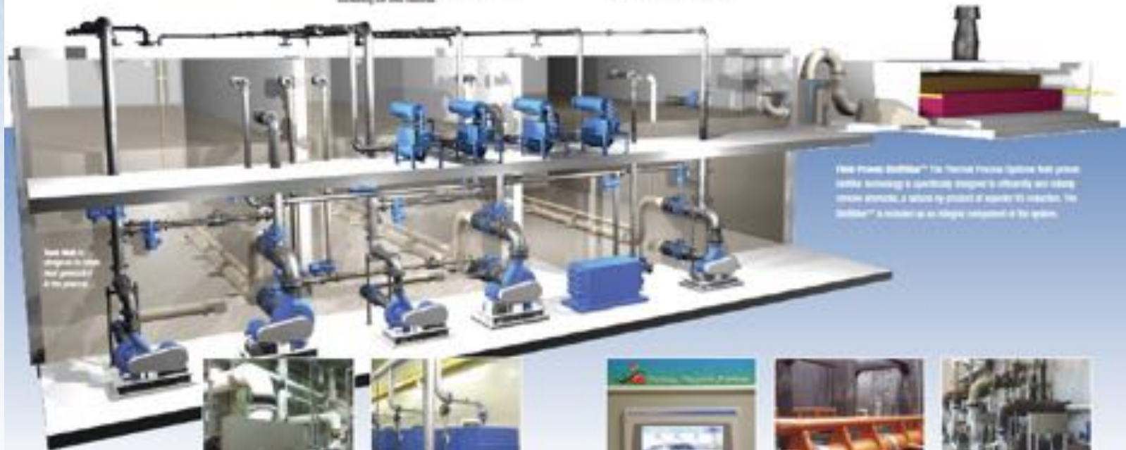
Pump Gallery — Douglas, OK. 100,000 lb. system. Pump mounted at grade for all pump access.
