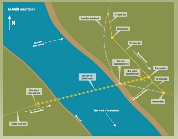
The design of the permanent repair included increasing the siphon barrel diameter to 10" in order to alleviate the frequent surcharging that the 8" lines of the old siphon caused. Directional drilling was used to place the new siphon 15' below the riverbed. The new siphon outlet structure was relocated 50' back from the riverbank to reduce risks from future storm events.
