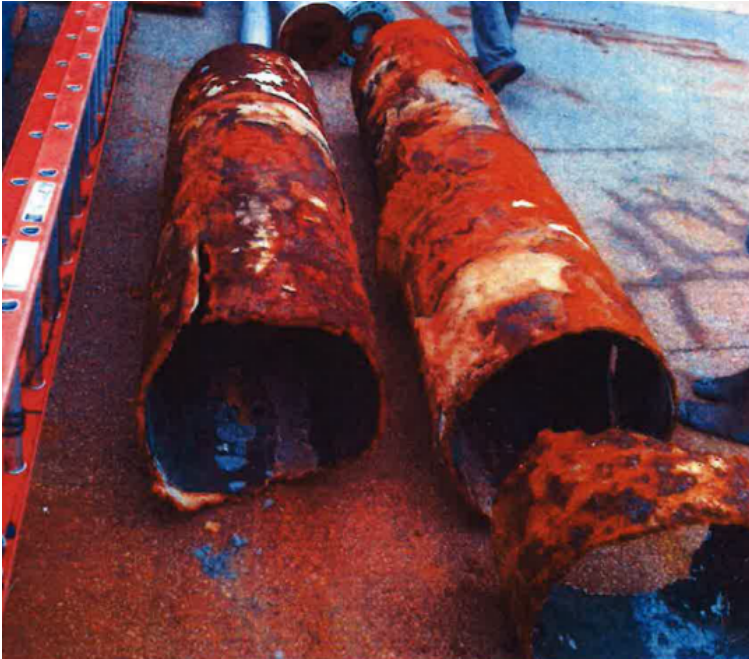
Perforation through DI pipe wall
