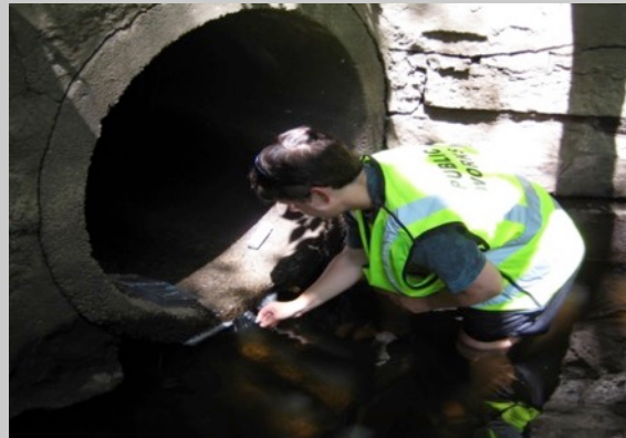
Outfall dry weather sampling
