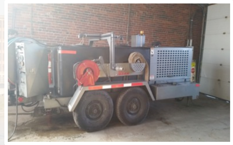
Lawrence Water and Sewer Division's Trailer Pipe Jetter
