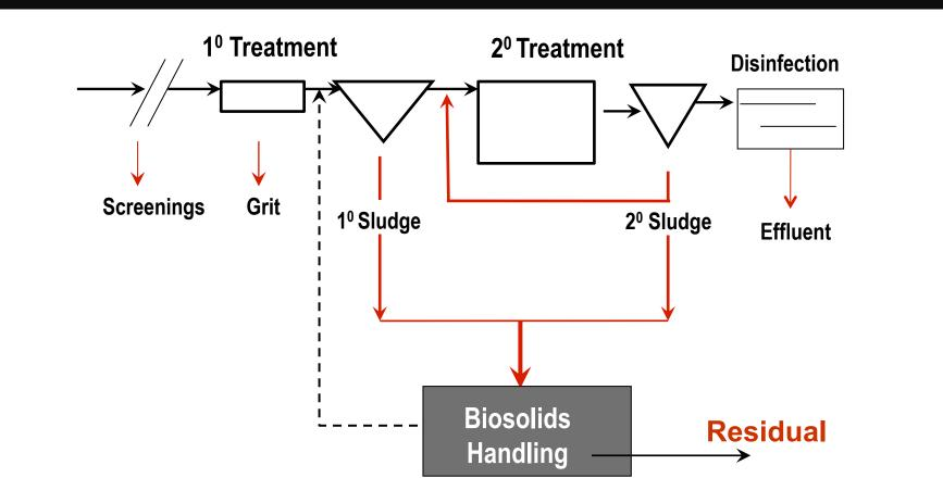
WRRFs designed for bulk carbon and pathogen reduction More recently, there has been a focus on biological nutrient removal > 84% of WRRFs facilities in USA have some form of biological treatment
