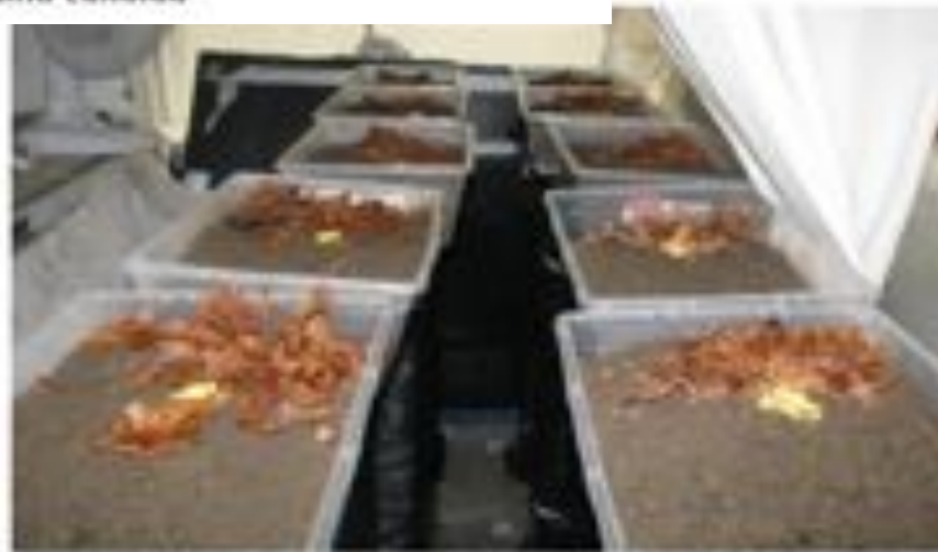
Figure 30: Feeding of Earthworms in Ryerson Long-Term Bioassay Chambers. Image shows the mating chambers atop the Evan's Boxes
