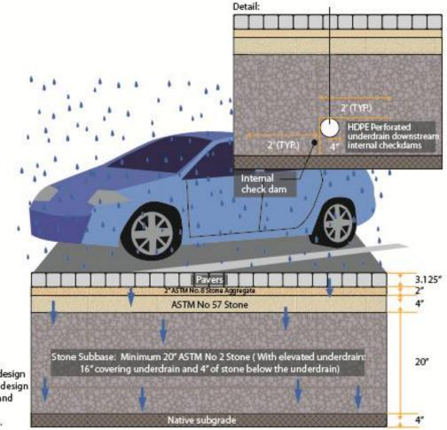
Please note: This design includes subbase design for cold climates and drainage for low permeability soils.
