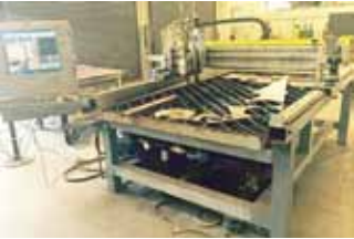
Building a precision cutting tool from salvaged parts enables the Village Creek Water Reclamation Facility (Fort Worth, Texas) to make the custom pieces it needs for repairs.
